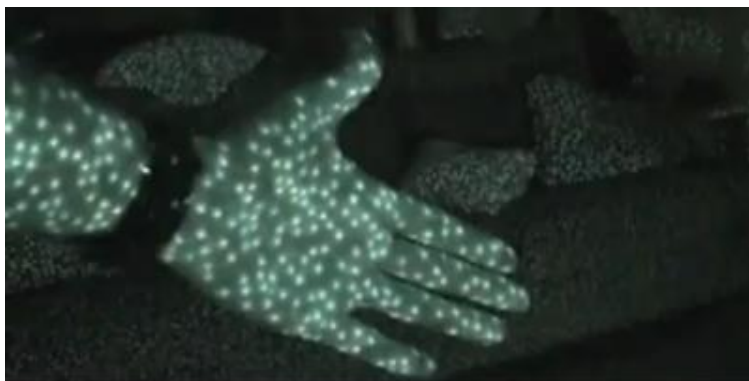
Figure 13 – Example of the structured light projected by a Microsoft Kinect device (source: Taylor, 2011)
