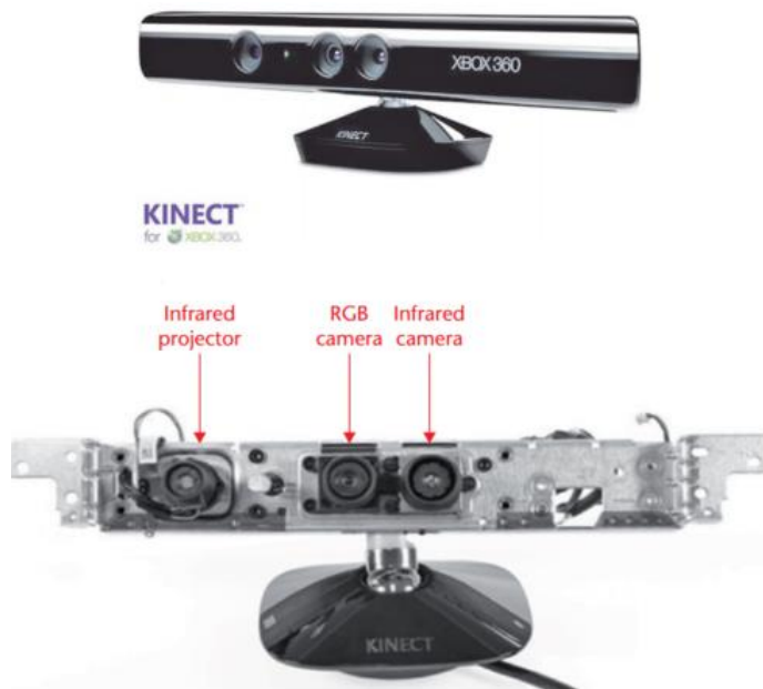
Figure 12 – Microsoft Kinect teardown showing the infrared projector, RGB camera and infrared camera (source: Zeng, 2012)
